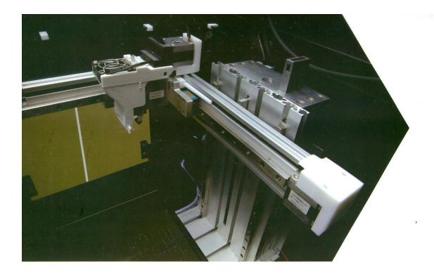
The X5 is a breakthrough in 3D printing, designed from the ground up for low-volume manufacturing. Capable of automatically feeding up to 12 print beds onto its build plate and reloading during printing, it provides a continuous 3D printing experience.
